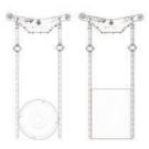
BlinkTroll can be configured to your choice of target. With a carrying capacity of up to 6 kg, the BlinkTroll can be used with a steel target, cardboard cutouts or archery targets.
